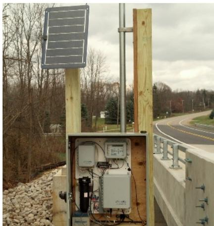
*A stream gage deployed by the USGS Michigan Water Science Center, Lansing Field Office.*
